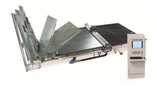
The totally new and also revolutionary conception of the REV tables' series breaks the traditional mould of the cutting machines, placing this range of machines at the top in technology, performances and design. For a dynamic response of the axes the operational and control system of the machine is completely "digital", thus enabling a high control of the cutting speed and the cutting accuracy.
