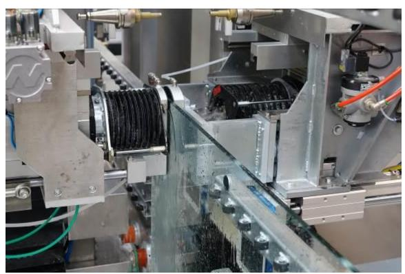
It is made up of two electro-welded steel vertical rods, supporting the spindles (Y-axis) sliding on ball guides and pads. The movement of the heads is by means of two ball screws with a brushless motor. The horizontal translation of the glass constitutes the X-axis: the sheet is moved by the motorized rollers.
