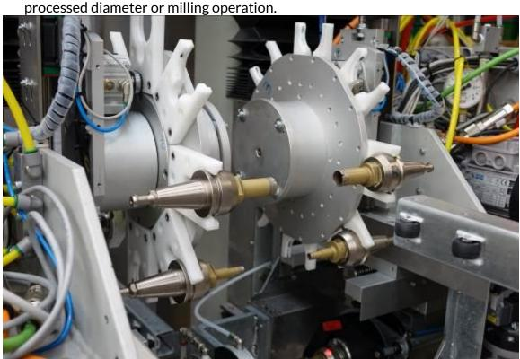
Milling will be performed while the glass is in a fixed position in order to achieve better grinding quality and higher grinding speed.
