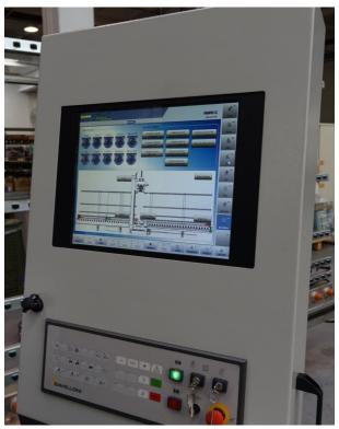
The control device combines a professional numerical control with the convenience of a PC working in Windows® (Microsoft) environment.
