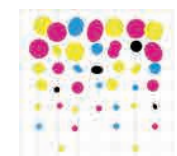
Gapping or overlapping occurs. The image quality is rough and the edges are blurred.
