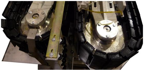
The opening is made by a mechanical device motorized and controlled by the NC. The VE 350 series machines use a **patented** conveyor, sliding on high precision ground steel guides without the aid of ball bearings.
