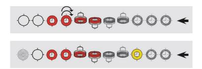
If a brilliant finish is required, a cerium oxide polishing system consisting of: tank, pump, mixer, filter and connecting pipes is available as an option. This system requires the use of a felt wheel in position 11.
